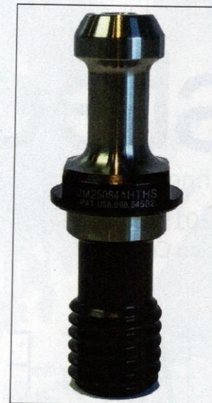
JMPP's High Torque knob is longer and reaches the cross section of the threaded bore. As a result, the thread engagement region of the toolholder is increased, the cross-section is larger, and the order to resist deformation is increased, increasing rigidity and
